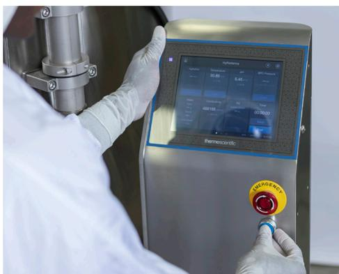
Figure 6. Pushing the power on reset button
