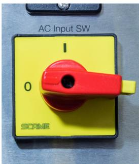
Figure 3. Main power switch, shown in the “Off” position
