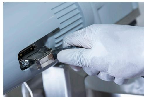
Figure 4. Connecting the power cable to the motor
